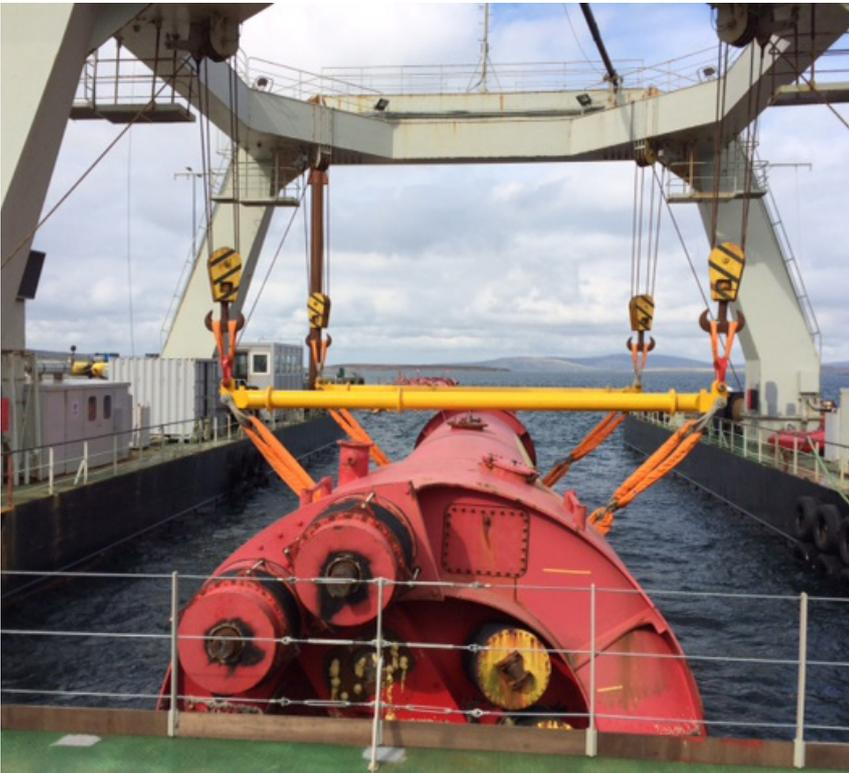
Lifting a 300 tonne wave energy device out of the North Sea is no easy task, so when the energy support services company, Green Marine was asked by Wave Energy Scotland to decommission the equipment, the company relied on Modulift Modular Spreader Beams to help with the job.
